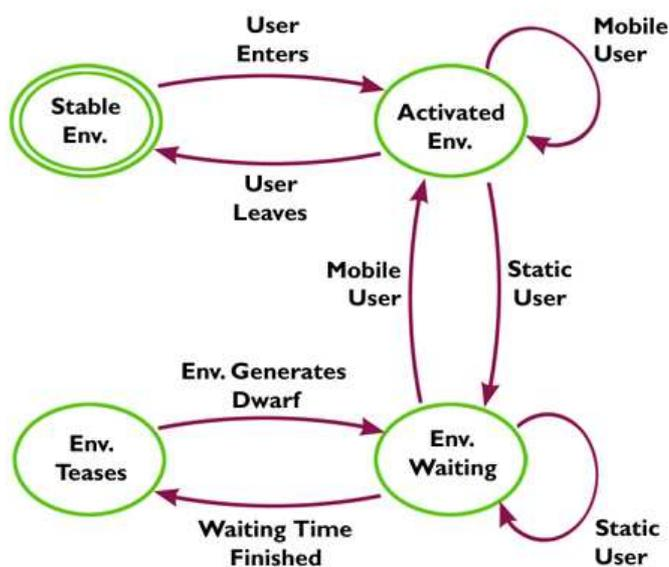
Figure 5: example of Fullaraca, one of the automata developed that describes the states that the model can have as a function of user interaction.
