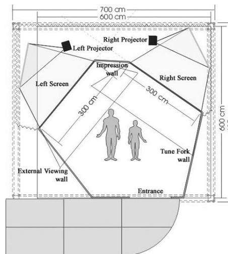
Figure 2: Plan view of the physical shape of MEDIATE: an irregular hexagonal space provides a good set up for free-roaming full-body interaction.
