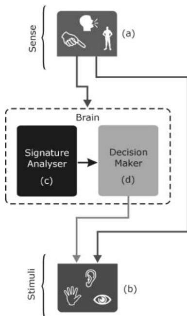
Figure 1: Block diagram of the modules of the system: (a) sensed inputs from user (sound, touch & gesticulation), (b) stimuli (output of the system to user: sound, vibration & visuals), (c) Signature Analyser, (d) Decision Maker.
