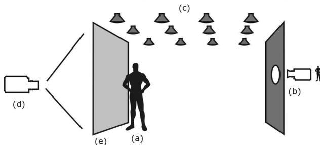
Figure 3: Artificial vision system for capturing gesticulation and position of the user. (a) the user's image is captured by cameras (b) behind the environment's walls. The environment and user are lighted by near-infrared lights (c) such that the camera can clearly capture the user, without disturbing the correct visualization of images projected by the rear projection (d) on the screens (e).
